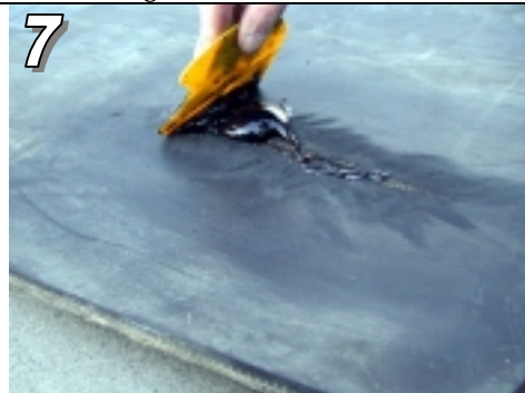
7 Apply Eli-Flex to the topside of the repair. Use a spatula or any straight edge tools to force the Eli-Flex into the repair opening. Recess the repair slightly to reduce contact with the belt cleaner
