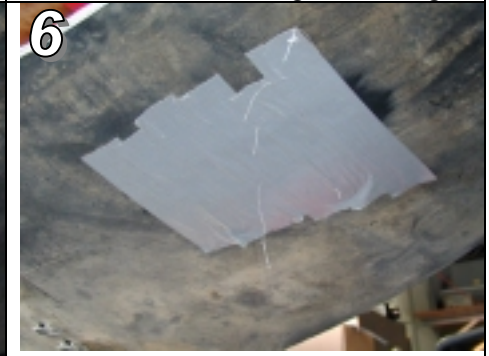
6 Cover the underside of the belt with industrial tape to prevent the opening from being forced through the opening.
