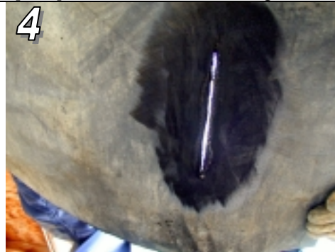
4 If the tear has left a large hole it may be necessary to roughen the underside of the belt. If possible skive the bottom layer at 45° and roughen the surface
